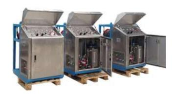
Emergency Shut Down Control Panel is designed to generate signal to pneumatically control the ESD system controls the hydraulic safety valve on the test tree and on the well head wing valve and allows manual or remote closure in response to any equipment failure upstream of the choke manifold such as pipe leaks, equipment malfunction, fire or any emergency that may occur during the operations.
