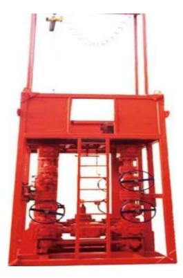
Dual Pot Sand Filter is skid unit improve well analysis during testing operations through the effective removal of sand and other solids from the well effluent, which working pressure is 5000psi, 10,000psi and 15,000 psi.
