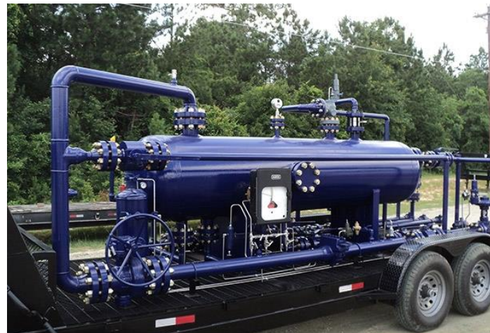
30"OD X 10' L X 2160 PSI 3 PH Horizontal Test Separator
