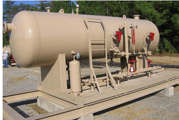
54"OD X 15' L X 285 PSI 3 PH Horizontal Production Separator
