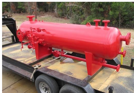
30"OD X 10' L X 1440 PSI 3 PH Horizontal Production Separator
